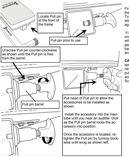
First, locate the Pull pin at the front of the frame under the main bench pad. To operate, turn the pin counter clockwise until you are able to pull the pin against the spring.
